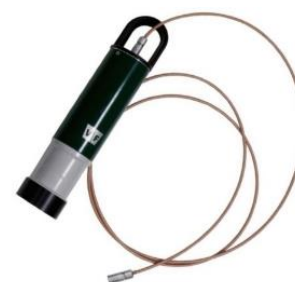
GD-52 detector with stabilization source
